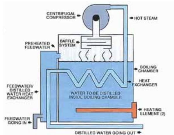
Figure 2 Diagram of a Typical Vapor Compression Distiller, from Ref. 2
